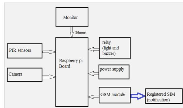
**Fig. (1) : Block Diagram of ATS-IOT**
