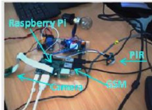
Fig.(2): ATS-IoT- Raspberry Pi, GSM, PIR
