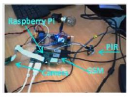
Fig.(2): ATS-IoT- Raspberry Pi, GSM, PIR
