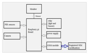
Fig. (1): Block Diagram of ATS-IOT
