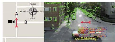
Fig. 5—Extracting the Direction of Motion and Coordinate Transformation
