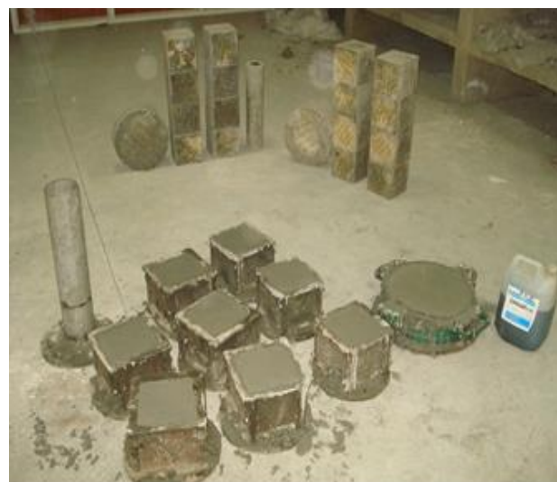
Fig 1: Casting of Concrete cubes
