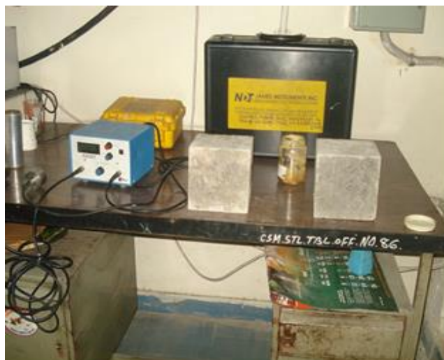
Fig 3: UPV Testing in Progress
